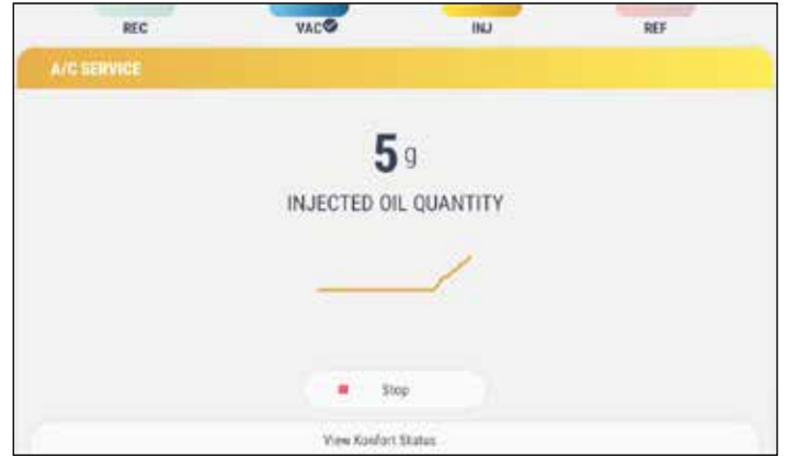
«Oil injection» phase: the system injects the correct amount of oil in the vehicle system to lubricate it.
